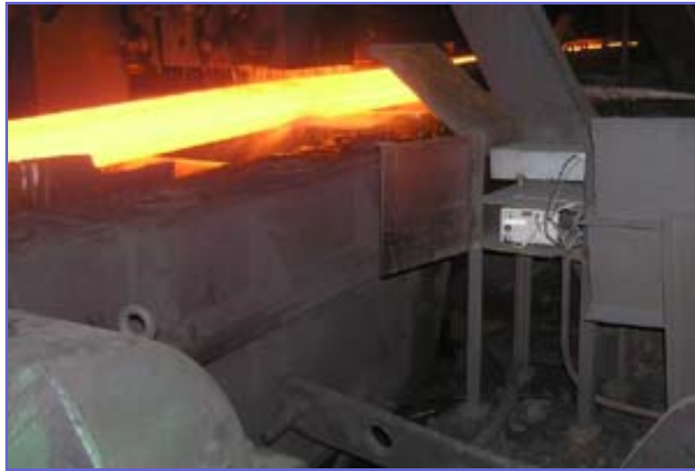
Fig.5 ICV controlling billet cutting machine
